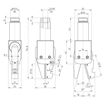
A = connection port B = fixing thread C = sensor fixing hole
