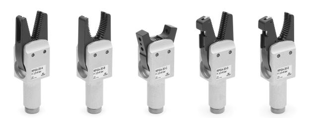
Thanks to a piston with a size of 20mm and to the direct transfer of the force from the piston to the fingers, Series RPGA guarantees a strong and a safe Their technical features ensure a high gripping force and make these grippers particularly suitable in the removal of injection molded items. The surface treatments on each metallic part make this series very wear resistant.
