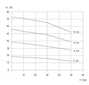
The total gripping force has to be calculated as follows: Total  $Fc = Fc \times 2$
